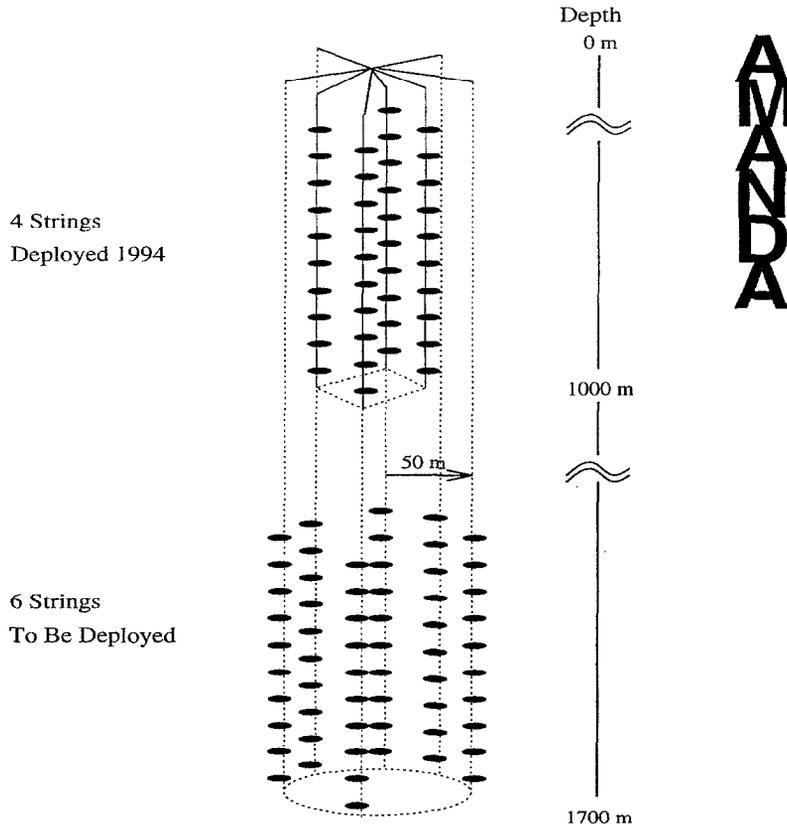
Fig. 28. Diagram of the AMANDA neutrino detector [338]. The final configuration may differ slightly from that shown here.
