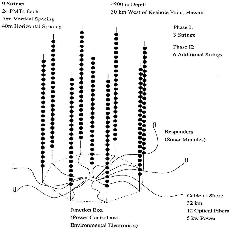
Fig. 27. Diagram of the DUMAND neutrino detector [337].
