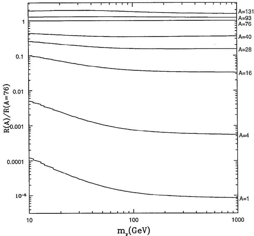
Fig. 26. Event rate (per kg of detector) for scalar-coupled WIMPs in a detector composed of nuclei with mass number  $A$  scaled by the rate in a  $^{76}\text{Ge}$  detector as a function of WIMP mass  $m_\chi$ . Threshold effects are neglected. (From Ref. [301].)
