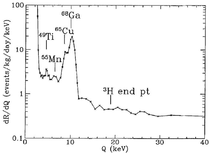
Fig. 25. Measured gamma-ray background in an underground high-purity germanium ionization detector (data acquired by the UCB/UCSB/LBL experiment at Oroville [307, 420]). Various gamma-ray lines are identified, as is the end point of the broad tritium spectrum. The rapid rise at low  $Q$  is the electronic noise. Compare with the potential WIMP signals shown in Figs. 23 and 24.
