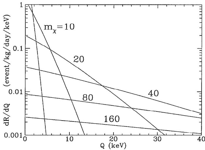
Fig. 23. Theoretical differential event rate for WIMPs of various masses hitting a germanium target. WIMP masses are labeled in GeV. An arbitrary cross section of  $\sigma_0 = 4 \times 10^{-36} \text{ cm}^2$  was chosen with standard values for the other parameters. Compare these curves with a typical experimental gamma-ray background shown in Fig. 25. Note the rate axis scale is 100 times *smaller* than in Fig. 25, and the cross section chosen is very high for neutralinos (see Section 11).
